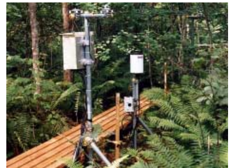
Micrometeorological measurement instruments at forest floor
