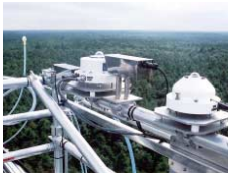
Radiation measurement instruments installed on the top of tower
