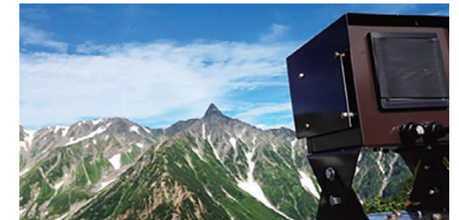
Time-lapse camera monitoring Mt. Yurigatake installed at Hyutte Nishidake, Japanese Northern Alps
