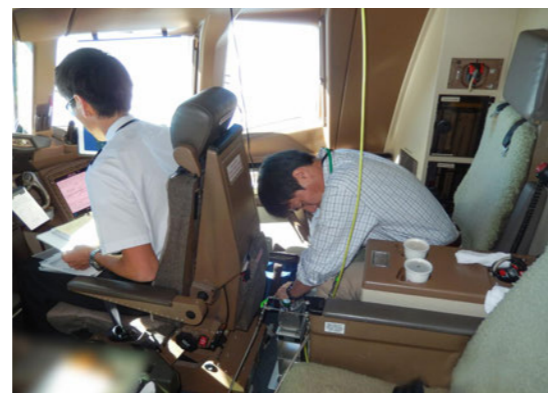
Sampling air by MSE (Manual Sampling Equipment) in the cockpit (by courtesy of Japan Airlines). Picture taken after full confirmation of flight safety.)
