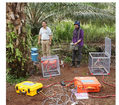
Measuring site for soil CO 2 and CH 4 fluxes in Malaysia
